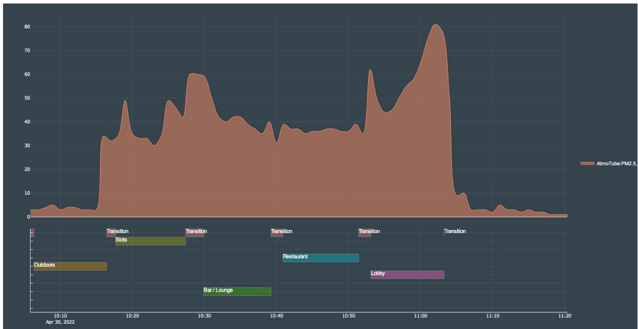
Supplementary Figure 1. Example time series of personal PM 2.5 concentrations in µg/m 3 measured by an AtmoTube PRO air monitor during a casino visit (spline fit 1-minute readings). Locations visited are shown as bars below the time series. The locations and other observational data were recorded in real-time using a custom “Casino Logger” mobile app.
